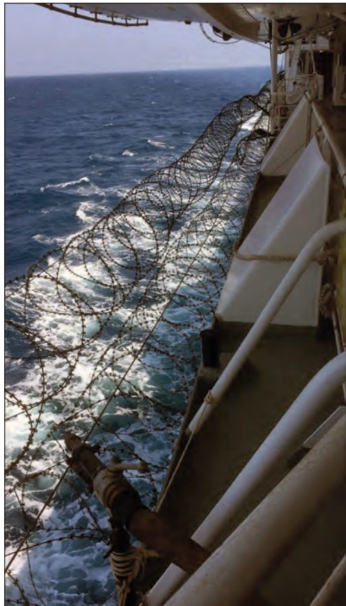
Plate 1. MV Minerva dressed in rolls of razor wire and numerous water cannons as part of the defence against the threat of Somali pirates, April 2015. © Robert L Flood
