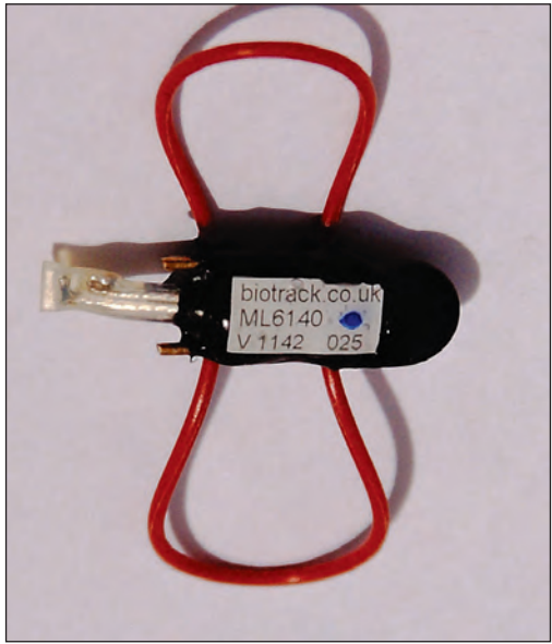
Plate 1. Biotrack Geolocator model ML6140 which was fitted on Cyprus Wheatears Oenanthe cyprica with an O-ring harness. © Alan Crabtree
